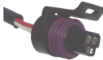
Fig.3: The terminals in the shafts of the connector
